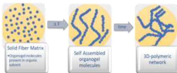
Fig 2(b): Gel formation mechanism by Solid Fiber matrix
