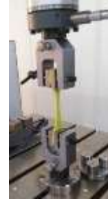
Figure 4: Measurement of tensile strength by Universal testing machine
