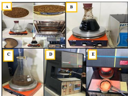
Figure 1: (A) Preparation of rice husk ash; (B) Rice husk ash in NaOH; (C) Titration with H 3 PO 4 ; (D) Calcination furnace; (E) Resultant silica
